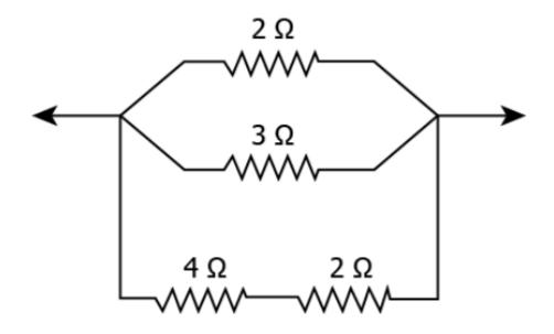
What is the net resistance between the two points in the circuit?
